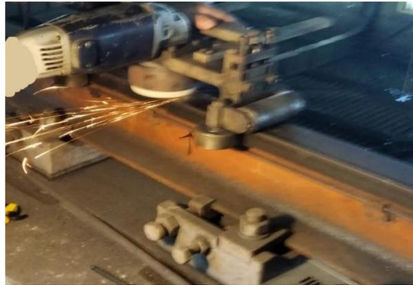
**Fig. 6.** Abrasive treatment of deposition areas
