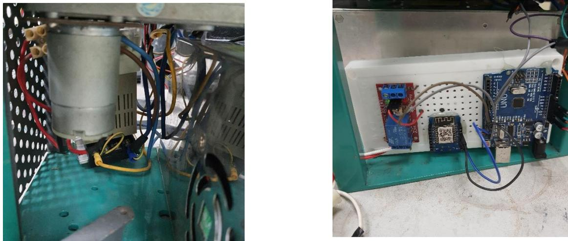
**Fig.8.** Electric parts location. (a) DC gearmotor, (b) Electricity board
