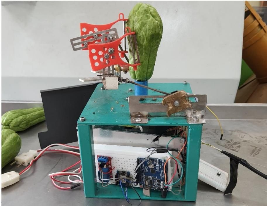
**Fig. 10.** Completed prototype of chayote peeling machine.
