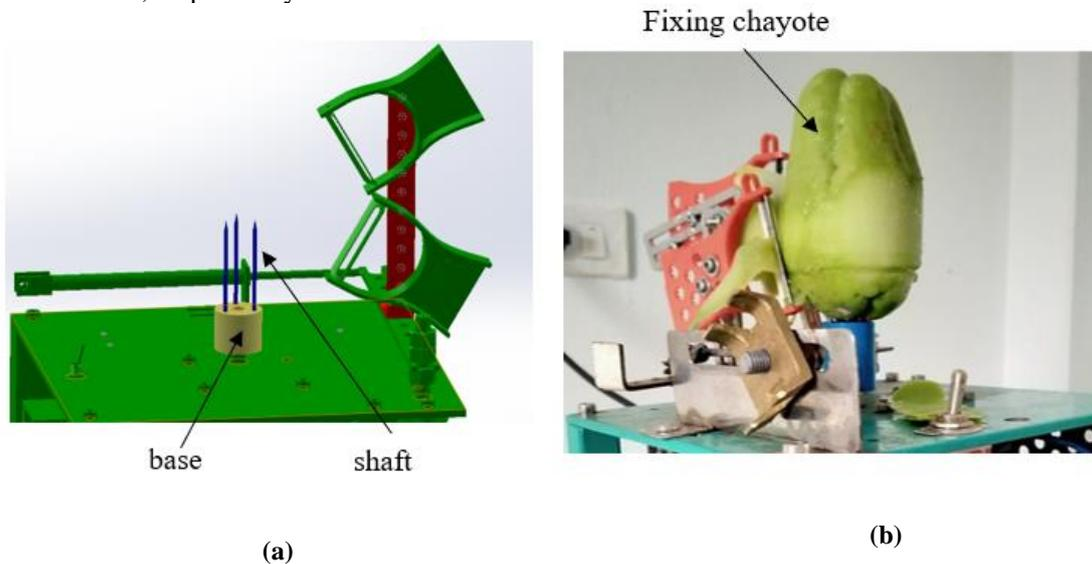
**Fig.3.** Rotating shaft with chayote fixing. (a) CAD model; (b) manufactured chayote peeling machine.
