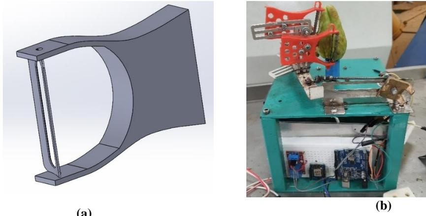
**Fig.6.** The cutting tool. (a) CAD model, (b) Cutting tools locating on the machine.
