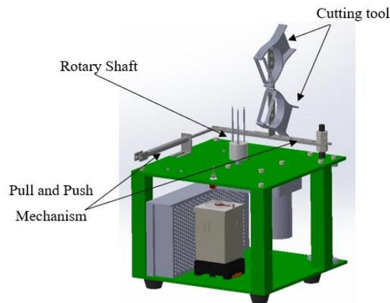
**Fig.2.** Machine Model.
