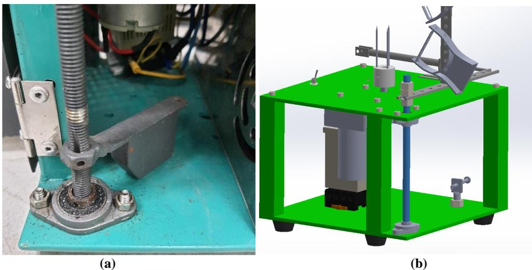
**Fig.9.** The spindle and lead screw nut.
