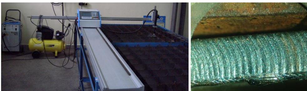
Fig. 1. A system of the type SteelCut – L and specimen surface made of steel C45 after gouging
