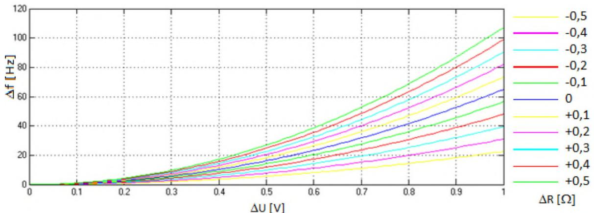
**Fig. 2.** Modification of the output frequency  $\Delta f$  depending on the amendment to  $\Delta U$  and  $\Delta R$ .
